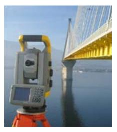
STRUCTURAL MONITORING USING ATS
